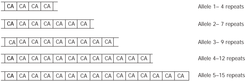
Fig. 16.5 Microsatellite marker (CA repeats). A number of alleles are possible. When the DNA segment containing CA repeats is amplified by PCR and the product is electrophoresed, the size of the band will vary depending on the number of CA repeats.
